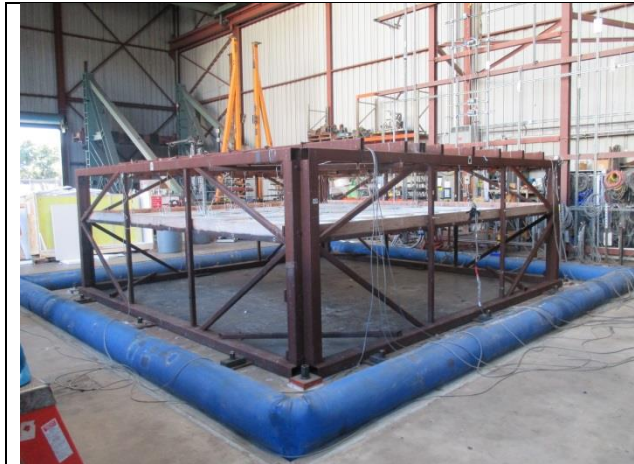
Photo 1: Test Frame with Claro Installed
